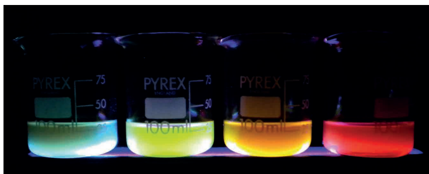
Samples of CPNs™ excited with 365 nm light
